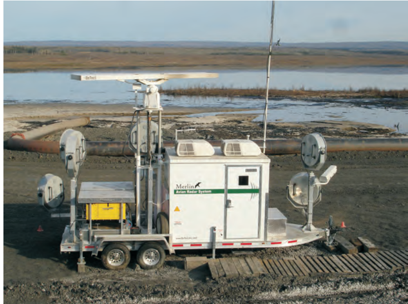
TOP: MERLIN detect & deter system installation at oil tar sands processing facility waste pond in northern Canada providing migratory bird control; networked system includes two self-contained master radar trailers & two satellite deterrent unit trailers.
