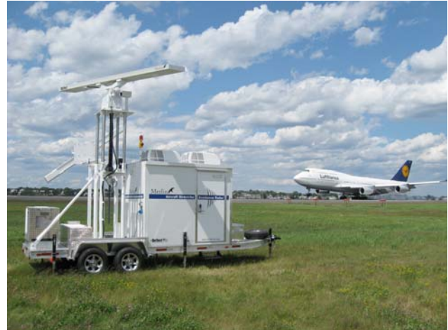
MERLIN Aircraft Birdstrike Avoidance Radar at Logan International Airport, Boston, Massachusetts, USA in July 2009.
