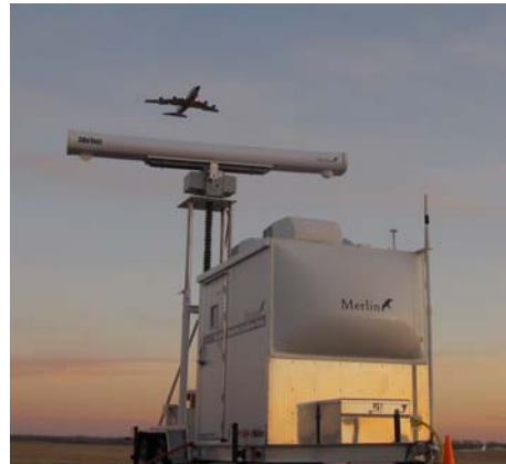
The MERLIN Aircraft Birdstrike Avoidance Radar System provides real-time detection and tracking of hazardous bird activity with automatic birdstrike risk warnings.
