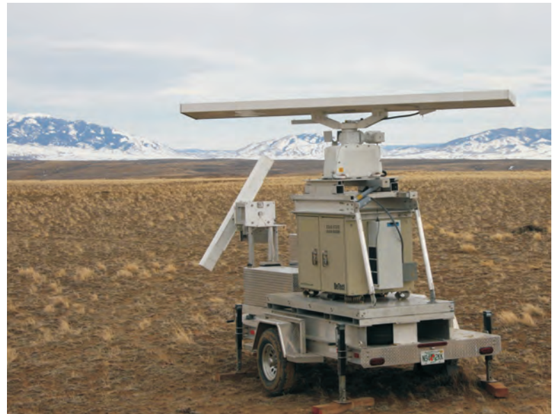
Lower photo: Mobile off-road HARRIER BSR 3D ultralight surveillance unit with Satcom remote data display & control..
