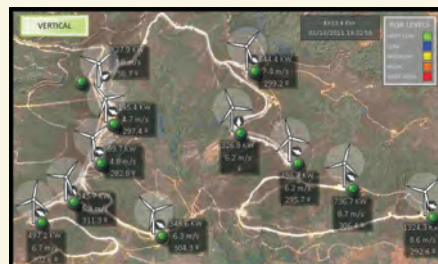
MERLIN SCADA-R interface for raptor mitigation using turbine centric model that idles individual turbines when proximate risk is detected; each turbine is assigned a color-coded risk value (El Pino wind farm, Spain)
