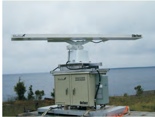
The SS-pe skid unit is designed to operate with standard commercial off-road lifts for access to remote areas and elevate the radar above obstructions such as tree lines.
