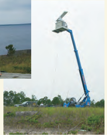
The SS-pe skid unit is designed to operate with standard commercial off-road lifts for access to remote areas and elevate the radar above obstructions such as tree lines.
