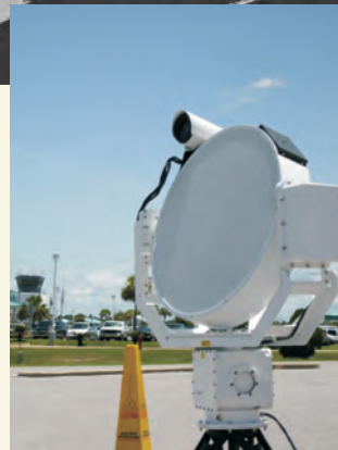
LEFT: Radar directed and activated Long Range Acoustic Device (LRAD) for raptor hazing. TOP: LRAD turbine coverage.
