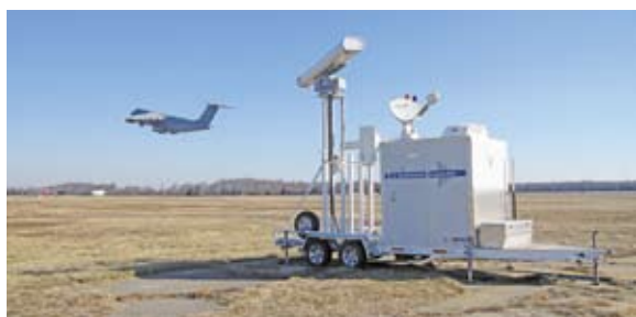
Airfield Avian Radar System with satellite data link allows operation at remote locations without network infrastructure. Typical Airfield systems use much larger and more powerful radars than can be employed by NASA for shuttle launch operations.
