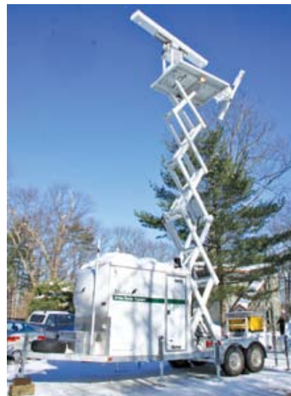
Mobile Avian Radar Systems are also used for environmental studies, monitoring bird activity at wind turbine sites and for other research needs. This particular system has a scissor lift to raise both the horizontal and vertical scan radars above the tree line or other obstacles on the ground allowing data collection in areas that would otherwise be impossible to use.
