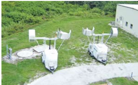
NASA Avian Awareness Radars at Kennedy Space Center, FL pointed towards Pad 39-A. For full redundancy during a launch a second duplicate radar system is available to the NASA Test Director for making launch decisions. The radars scan in both vertical and horizontal planes.
