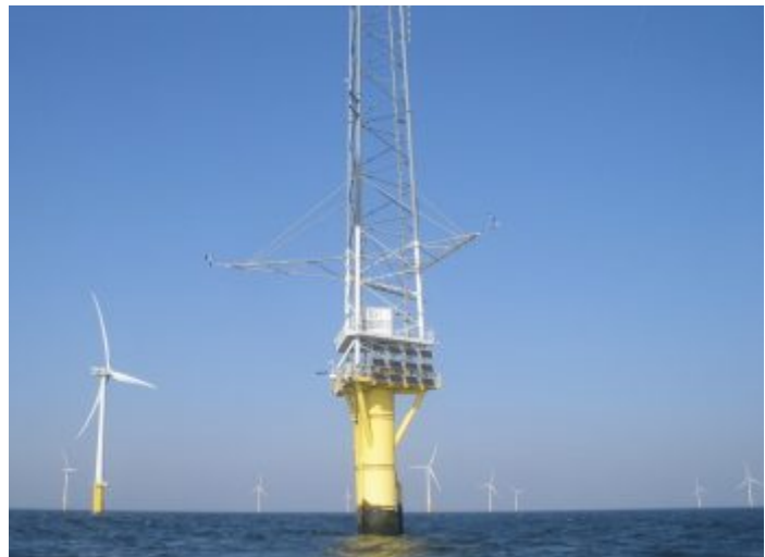
MERLIN XS2530e Avian Radar Monitoring system installed on monopole at the Nordwindzee wind farm in the Netherlands. The system is solar powered and fully remote viewable and controllable from shore and provides continuous monitoring of bird activity at the operating offshore wind farm, sending alerts to wind farm operators when risk events are detected.
