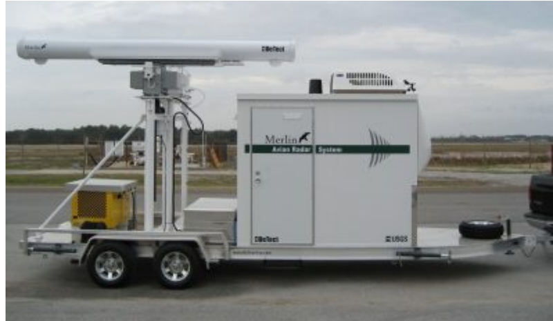
Standard 2007 MERLIN Avian Radar System Environmental Series build (side view) with radars and levelers retracted, stowed and locked for transport.
