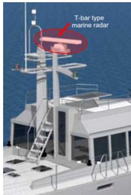
Example of T-bar type marine radar originally developed for maritime weather and navigation.
