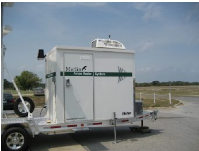
Standard 2007 MERLIN Avian Radar System Environmental Series build (door side of cabin view) with rain gauge (upper left) and keyless code-punch entry lockset.
