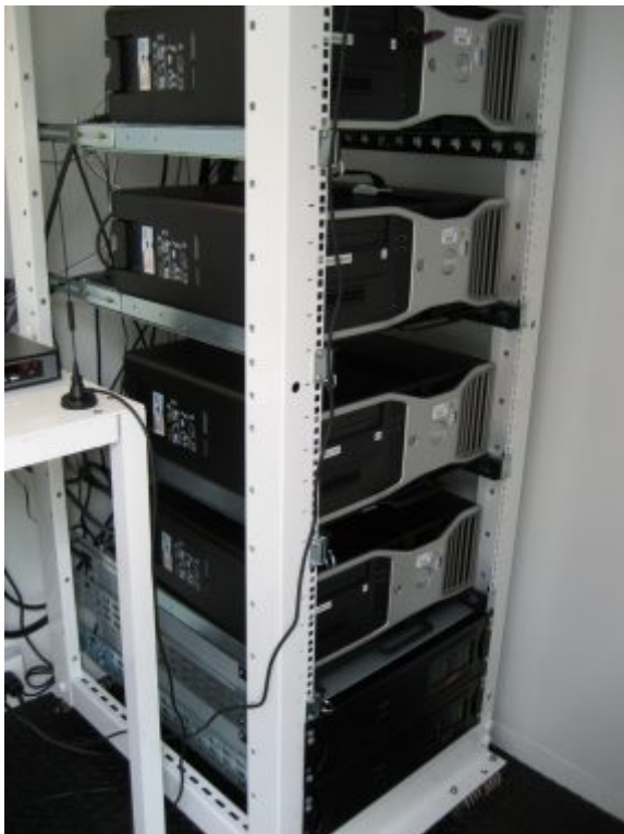
All system equipment is rack mounted in vibration and shock damped computer rack and housed in the environmentally controlled and monitored operator cabin.
