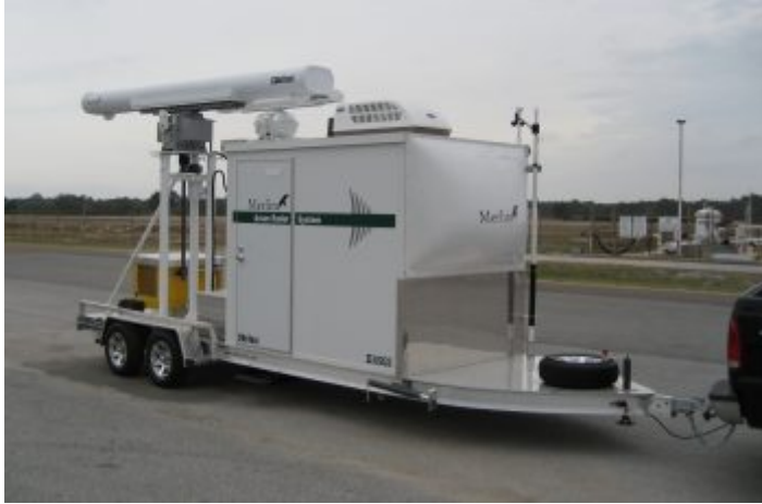
Standard 2007 MERLIN Avian Radar System Environmental Series build (front view) with MERLIN GPS/Compass mount (top right corner), weather system mast (retracted, top right corner), and optional aerodynamic nosecone.
