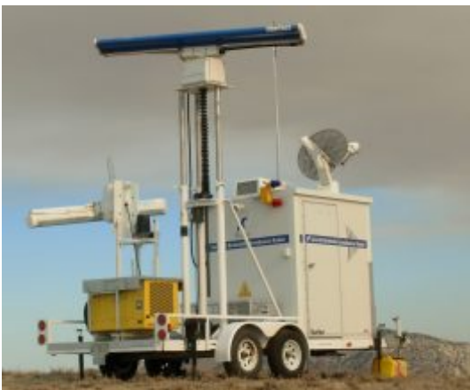
MERLIN Avian Radar System on Hoffman Wind Farm site, California during fall 2006 migratory survey.
