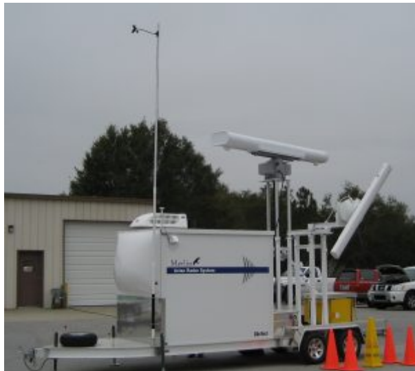
Standard 2007 MERLIN Avian Radar System Environmental Series build (back side view) fully deployed with radars and weather mast extended to operating positions.
