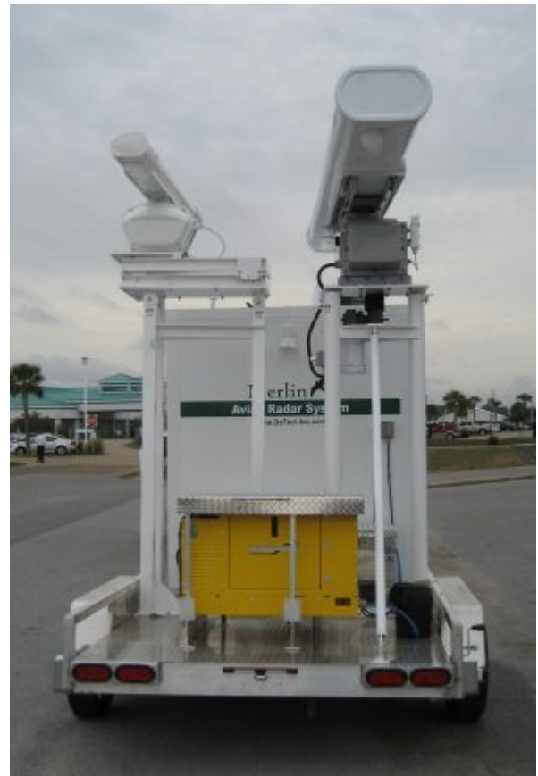
Standard 2007 MERLIN Avian Radar System Environmental Series build (front view) with radars retracted and locked for transport and optional on-board 6.5 kW diesel generator system.
