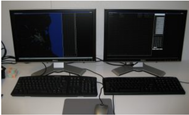
Typical dual radar system monitors with horizontal radar display on left and vertical radar display on right (from MERLIN Avian Radar installation at US Air Force Dover)
