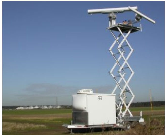
MERLIN XS2530ex Avian Radar System with extended 42 ft height tower (scissor) option purchased by the Government of the United Kingdom Central science Lab, York, England for wind farm surveys and migratory research.
