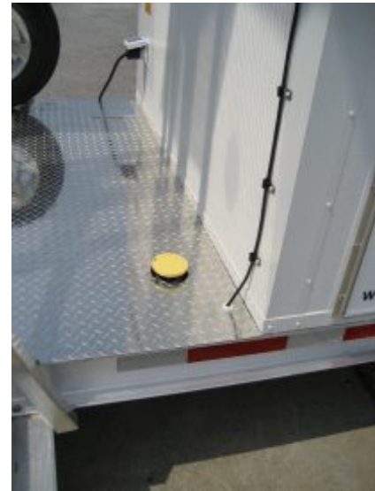
Close-up view of optional underdeck fuel tank and filler cap. Standard commercial power connection point shown in rear of photo.
