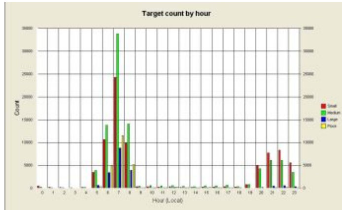
Chart of bird target count by hour of the day by size of bird for a 24-hour period generated by MERLINChart® data report software from MERLIN Avian Radar System database (note: peak activity periods for the dawn and dusk time periods for local wintering birds; data from USAF Beale AFB, California MERLIN XS2530m from January 2007).
