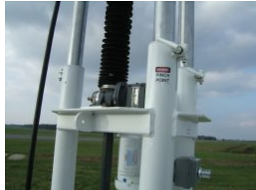
HSR radar tower with screw jack and key activated extension/retraction switch. :
