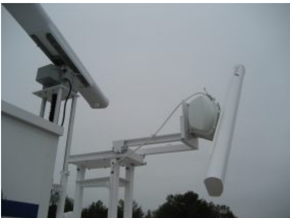
X-band VSR radar in operational position with slider extended.
