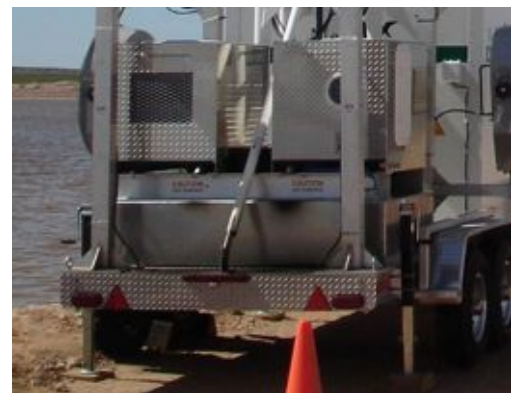
On-board dual diesel power system provides up to 500 hours of operation between generator service.
