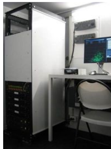
All electronic equipment is mounted in a environmentally controlled enclosures and vibration, rack mounted for portability and durability.
