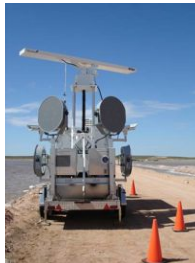
Mosaic MERLIN detect & deter system master radar unit, Carlsbad, NM, USA.
