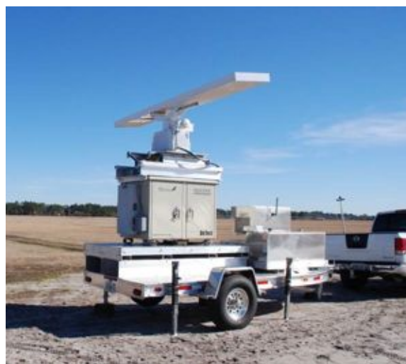
MERLIN is the only bird radar system that uses state-of-the-art solid state radars.
