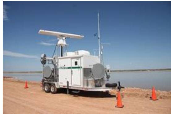
A Master MERLIN bird radar sensor unit provides 360 degree 3D bird detection and acts as the master controller for the overall MERLIN detect & deter system.
