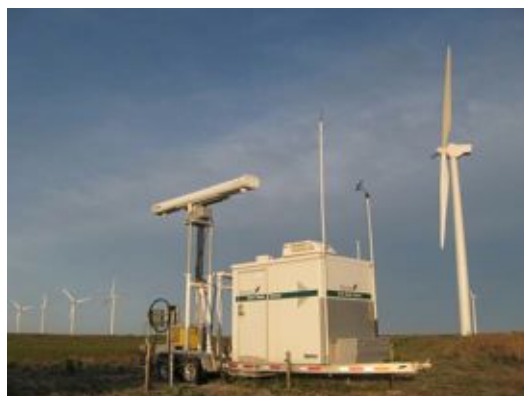
MERLIN avian radar system installed at the Gulf Wind I wind farm in Texas with MERLIN SCADA that allows the radar system to idle turbines when high bird mortality risk conditions are detected.
