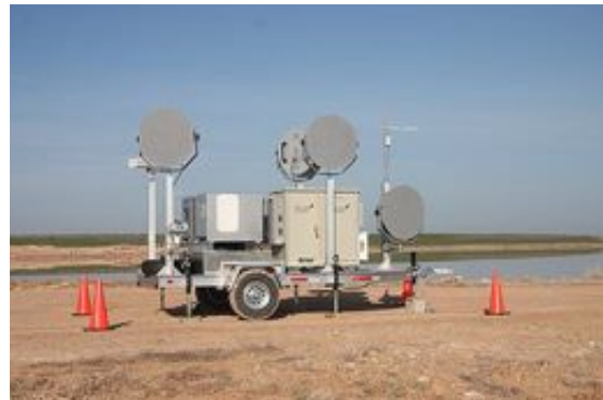
One or more Satellite Deterrent units with varied multiple zoned hazing devices are positioned to cover the control area and are remotely activated by the master radar unit through a fixed or wireless network. (MERLIN BCRS system installed at Mosaic Potash, Carlsbad, NM, USA)
