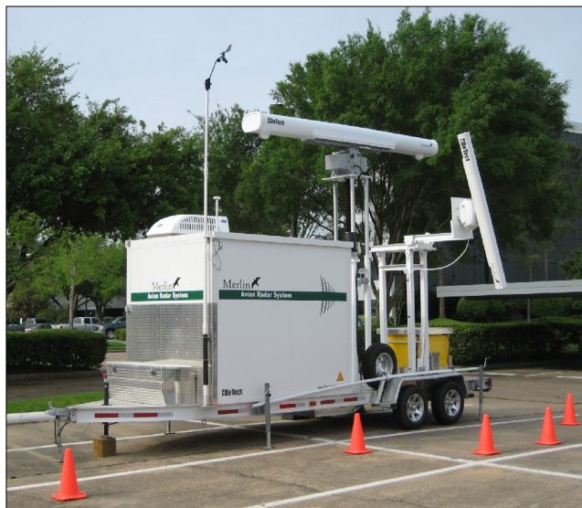
Figure 1: Typical commercially available avian radar system (DeTect MERLIN 1030e Avian Radar System, 2007 model).
