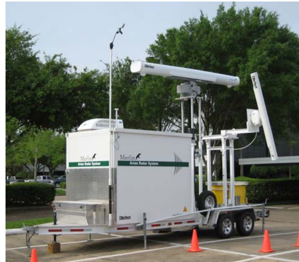
Figure 7: Advanced avian radar system developed by DeTect, Inc. of Panama City, Florida, model MERLIN XS2530e
