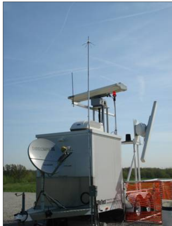
Figure 9: The MERLIN XS2530i Avian Radar System provides continuous 24-7 monitoring and comparative analysis of bird activity on and around the landfill property.
