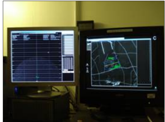
Figure 10: The MERLIN Avian Radar bird target data is displayed in real time at the radar on two display monitors.
