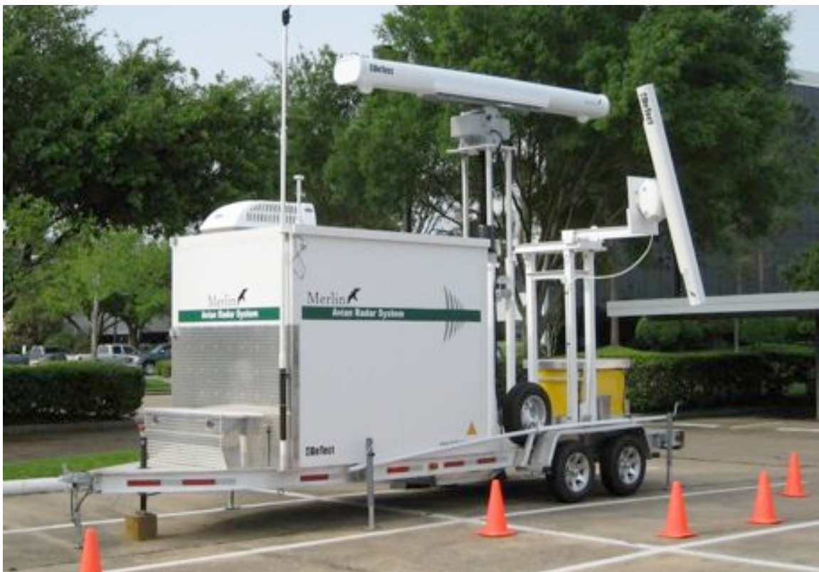
Figure 0: MERLIN Avian Radar System with dual radars
