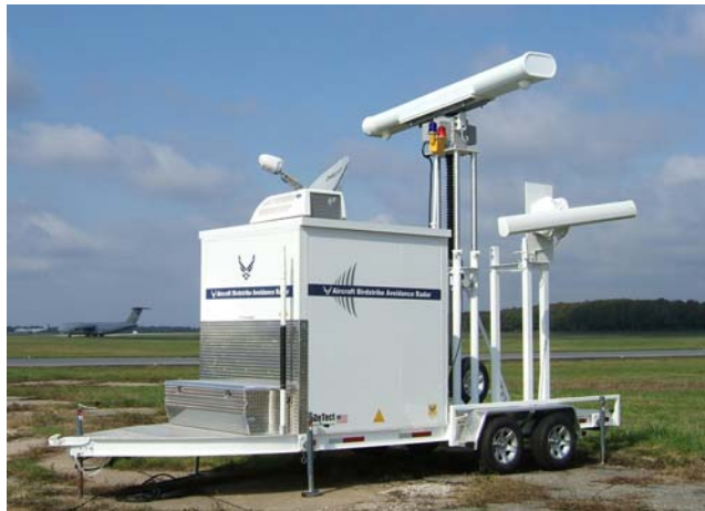
The standard production-model MERLIN Aircraft Birdstrike Avoidance Radar system is a dual radar unit that is installed at the mid-point of the runway; photo of MERLIN system installed and operating since 2006 at USAF Dover AFB, Delaware, USA
