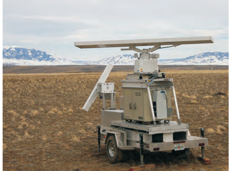
TOP: Portable off-road HARRIER 3D ASR for ultralight detection & border security.
