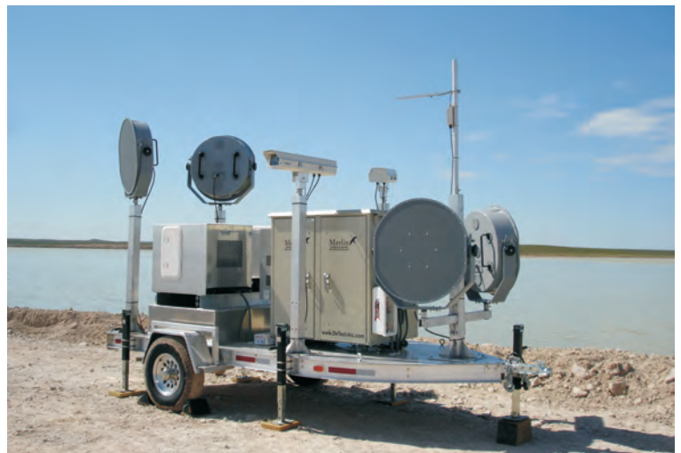
Satellite deterrent unit trailer with LRAD & laser units.
