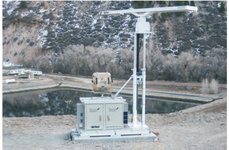
Skid-mounted single MERLIN detect & deter system for small gas processing facility waste pond resident & migratory bird control (Colorado USA).
